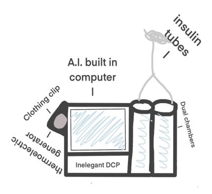
The current insulin pump is a one chamber pump; our idea is a dual chamber pump that uses Artificial Intelligence to manage insulin. In chamber one would be where the insulin is. In the second chamber would be the glucose for emergencies. No batteries or chargers are needed, the pump will be powered by body heat. Your body's heat is around 96-98, with that temperature your pump will be running successfully.
